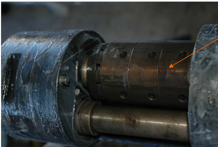
Main Thrust Bearing stack in excellent condition
