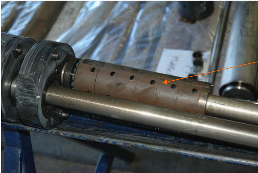
Main Thrust Bearing stack in excellent condition
